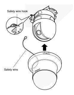
2 Mount this bracket on the camera with aligning the projection of the camera mounting bracket with "OPEN" of this bracket.
